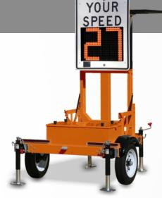
Frame Construction: 2" Steel Square Tube
