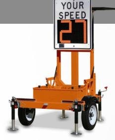
Frame Construction: 2" Steel Square Tube
