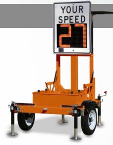
Frame Construction: 2" Steel Square Tube
